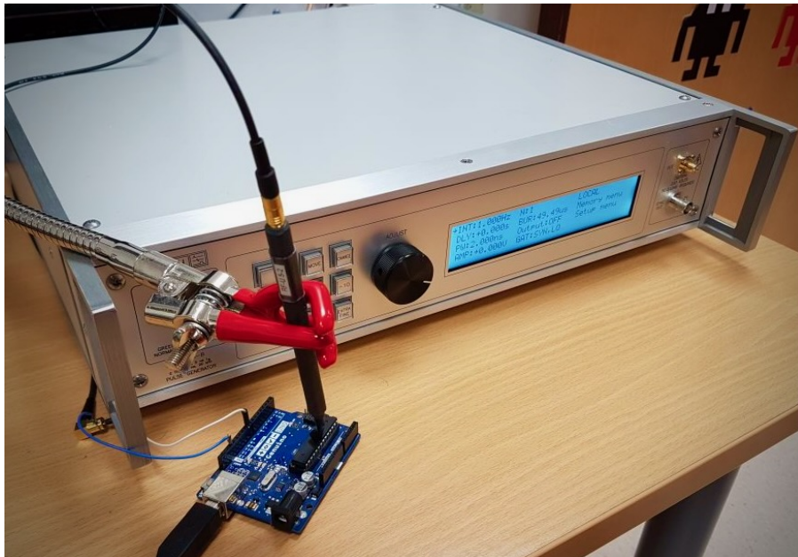
Figure 6.8: Depiction of a pulsed electromagnetic fault injection on an AVR microcontroller mounted on Arduino UNO board.
