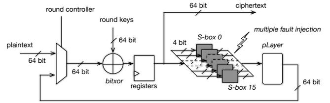
Figure 2. Parallel *Present* block cipher in FPGA.
