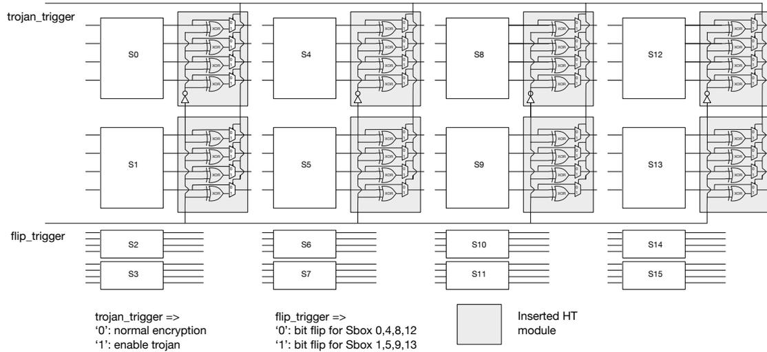
Figure 3. Trojans inserted into the signal paths after specific S-boxes.
